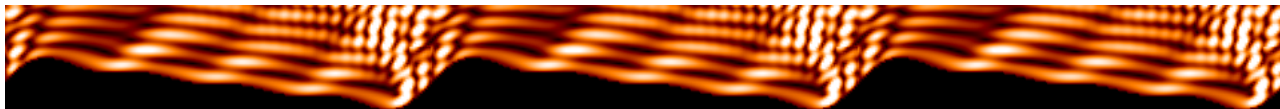
Figure 2.6.1: Depiction of the solution of the Wood-anomaly problem considered in Table 2.6.1. This solution resulted from a 0.9 sec. computation, which included the evaluation of the scattered field displayed.
